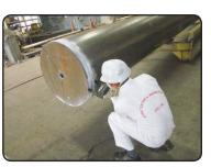
Magnetic particle Testing (MT) Surface and near surface inspection on welding joints.
