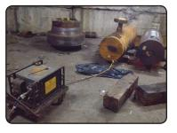
**Gamma Radiography Testing (RT)** Gamma ray inspection piping, pressure vessels, castings with Iridium 192, Cobalt 60 & Selenium 75.
