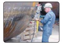
**Time of Flight Diffraction or TOFD**, is one of the most promising ultrasonic techniques for the examination of welds on pressure vessels in lieu of radiography; for pipe weld quality or crack detection and also weld root erosion. TOFD is a computerized ultrasonic system able to scan, store, and evaluate indications in terms of height (through wall thickness), length and position, with a degree of accuracy and speed never achieved with other ultrasonic techniques.
