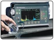
**Ultrasonic Testing (UT)** Thickness measurements and wall mapping for corrosion, flaw detection of piping, pressure vessels, structural parts.
