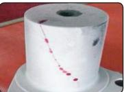
**Penetrant Testing (PT)** Surface breaking discontinuity inspection of welding, casting, structural members etc.
