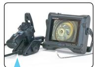
Our Video-probe is equipped with the latest technology in borescopes. A long fibre-optic cable illuminates the inspection area with light generated by a new state-of-the-art lamp in the Light Box. A miniature camera assembly in the viewing tip of the probe then converts the optical image into an electronic image. This image is carried back through the probe cable and displayed in the LCD color monitor. It allows the inspection of surfaces inside narrow tubes or difficult-to-reach chambers.
